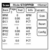
This page shows how injector duty cycle is monitored. First you configure RPM and the injector pulse width, then the IDC1 parameter calculates the duty cycle. You can use IDC1 & IDC2 to see if your fuel injectors are being over-worked. Scan this page & do a wide-open-throttle run, then click the "Info" button to see how high your duty cycle went. If it's over 90%, your injectors may need upgrading.
